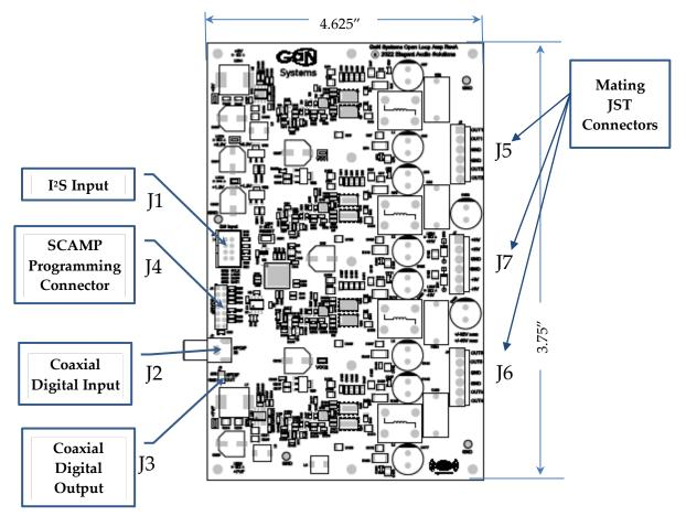
Figure 2 PCB Layout and Module Connections
