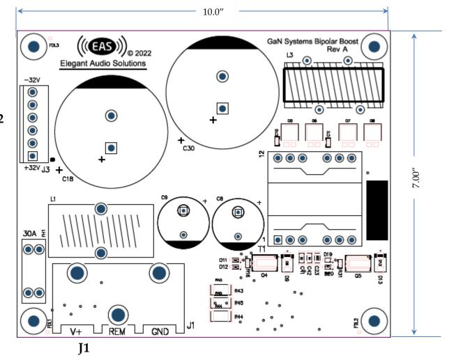
Figure 2 PCB Layout and Module Connections
