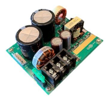
Figure 1 GS-EVB-AUD-BOOST-GS Evaluation Board
