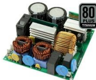
3kW bridgeless totem pole PFC
