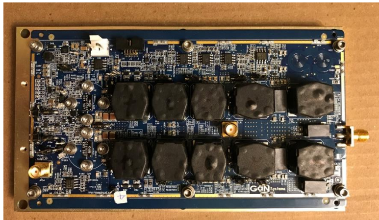
Figure 2 • Top side of GSWP100W-EVBPA Evaluation Board Assembly
