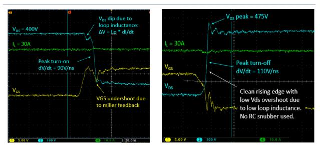
a) Hard switching turn-on 400V/30A b) Hard switching turn-off 400V/30A Figure 18 Double pulse test switching transient waveforms (GS66508T)
