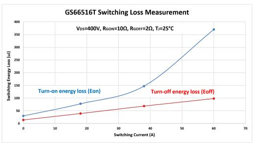
Figure 24 GS66516T Switching Loss Measurement (VDS = 400V, TJ=25°C)
