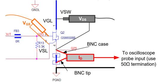
Figure 7 Recommended probe connection with current shunt
