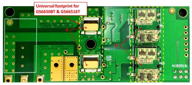
Figure 2 GS66508T/GS66516T-EVBDB2 bottom side (without heatsink)
