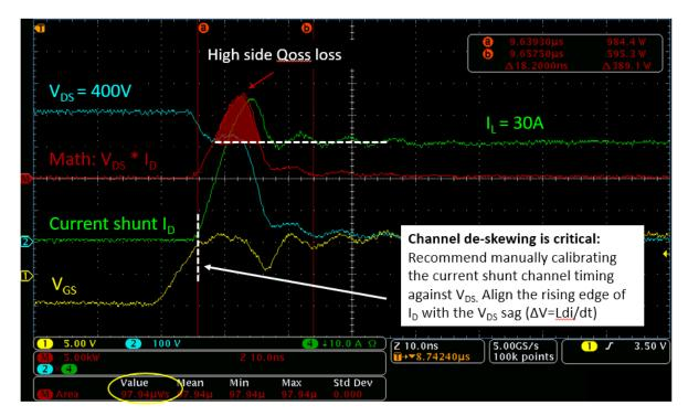
Figure 21 Turn-on switching loss measurement (Eon=98uJ, 400V/30A, TJ=25°C)
