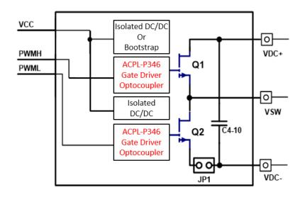
Figure 1 GS665XXT-EVBDB2 Evaluation Board Block Diagram
