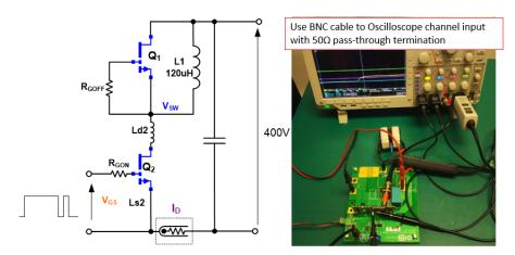
Figure 20 Eon/Eoff measurement and test bench setup
