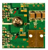
Figure 8 Location for case temperature monitoring
