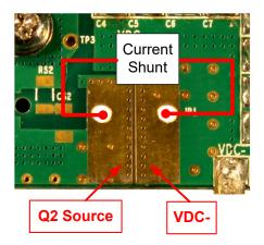
Figure 6 Recommended probe connection with current shunt
