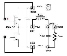
This standard half bridge configuration can be used in the following circuits :
