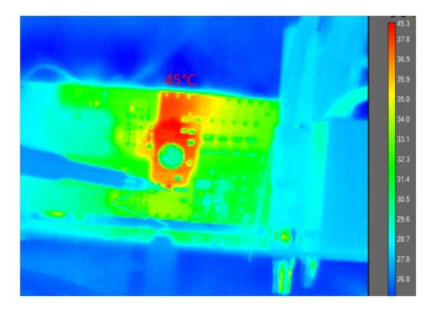
Figure 26 Thermal image (GS66508T, Pout=1kW)
