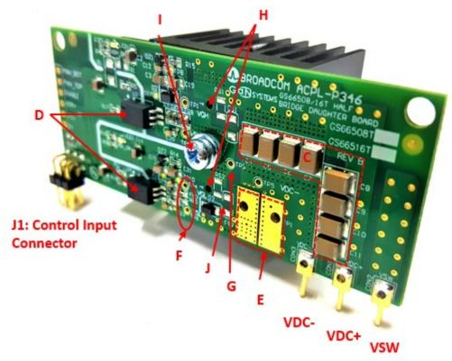
Figure 3 GS66508T/GS66516T-EVBDB2 top side
