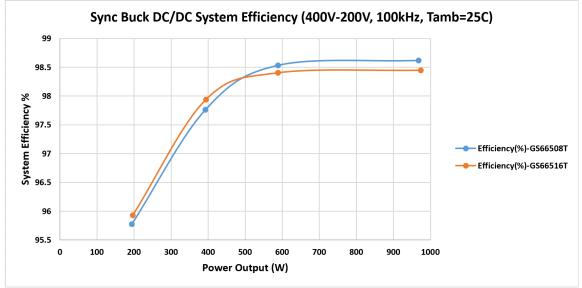
Figure 25 Synchronous Buck Efficiency and thermal measurement
