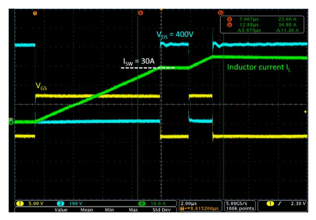
Figure 17 400V/30A double pulse test waveform (GS66508T)
