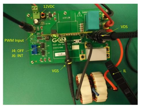
Figure 16 Double pulse test setup example
