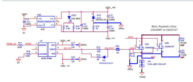
Figure 5 Gate bias and driver circuit
