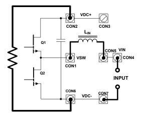
When the output becomes the input and the load is attached between VDC+ and VDC-, the board is converted into a boost mode circuit and can be used for:
