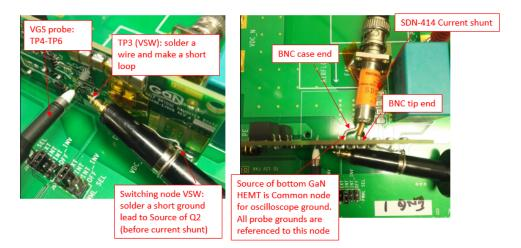
Figure 19 Eon/Eoff measurement probe connection with current shunt
