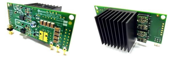
Figure 10: The daughter board assembly with heatsink attached
