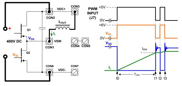
Figure 15 Double pulse test setup
