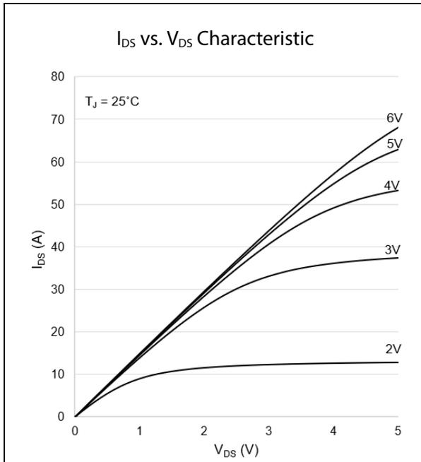
Figure 1: Typical  $I_{DS}$  vs.  $V_{DS}$  @  $T_J = 25\text{ }^\circ\text{C}$
