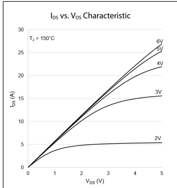
Figure 2: Typical  $I_{DS}$  vs.  $V_{DS}$  @  $T_J = 150\text{ }^\circ\text{C}$
