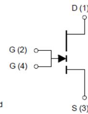
*The thermal pad is internally connected to Source (S pin 3) and substrate*
