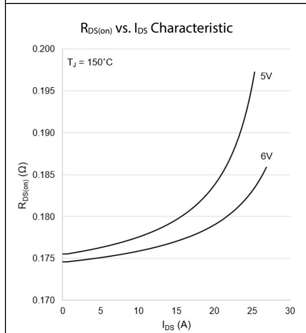
Figure 4:  $R_{DS(on)}$  vs.  $I_{DS}$  at  $T_J = 150\text{ }^\circ\text{C}$
