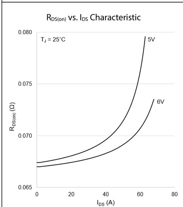
Figure 3:  $R_{DS(on)}$  vs.  $I_{DS}$  at  $T_J = 25\text{ }^\circ\text{C}$
