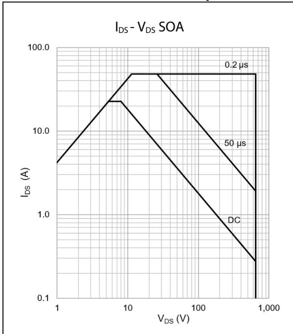
Figure 13: Safe Operating Area @  $T_{case} = 25\text{ }^{\circ}\text{C}$
