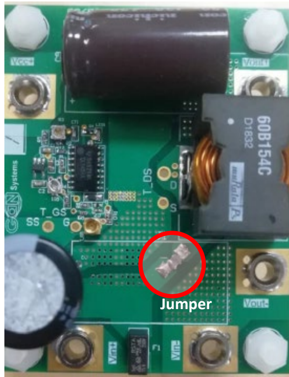
Figure 7 • Current Sensing Jumper Location
